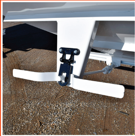
Butterfly Door Crank Easy-open operation with flip over locks.
